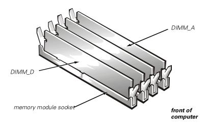
Figure 8-5. Memory Modules and Sockets
